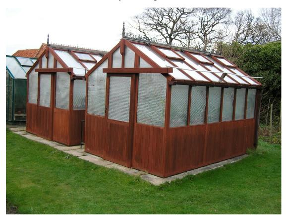
industry tests showed greater temperature variation (heat or cold) in metal structures through heat transfer in/out via the glazing bars whereas transmission through cedar was almost nonexistent. I concluded cedar construction rather than metal would suit my needs best, despite greater cost, a decision which has proved really beneficial. Wood is also easier to fix things and adapt internally. Both greenhouses are
